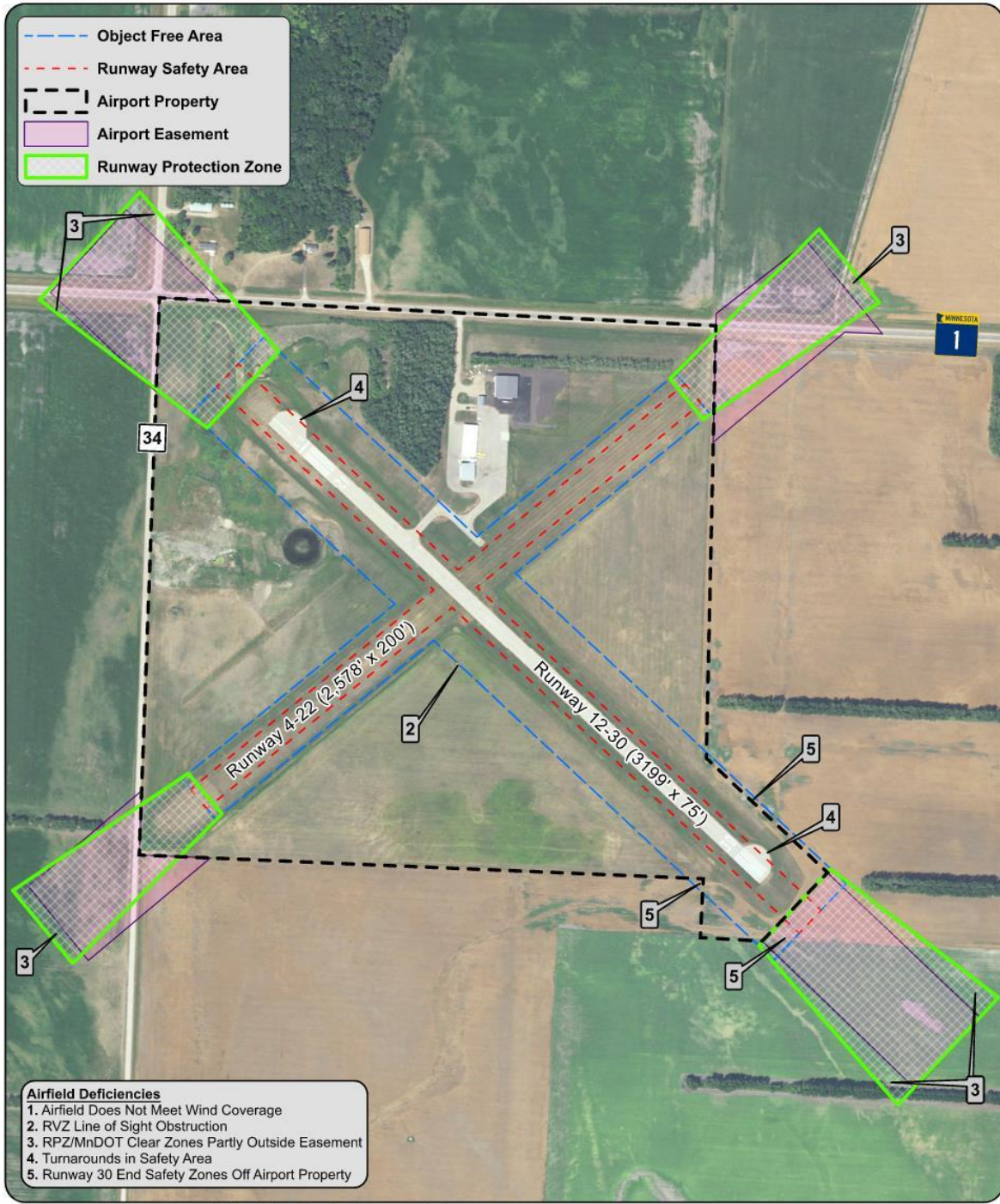
Figure 4-2 – Airfield Design Deficiencies
